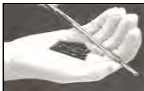
Each of these uranium fuel pellets contains the energy equivalence of about 1 metric tonne of coal.
