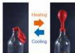
As the air inside the bottle is heated, the balloon begins to expand.
