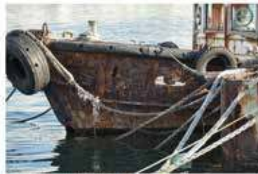
Rust on the surface of a ship.
