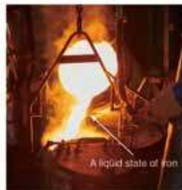
Iron starts melting at about 1500°C.
