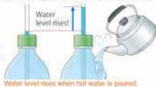
Water level rises when hot water is poured.
