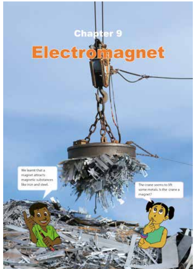
This picture is from the chapter heading of the textbook showing a huge electromagnet and attracted scrape metals attached to it.
